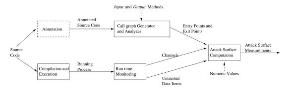
Figure 1: Attack surface measurement steps.
