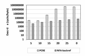
Fig. 4: Execution time (cycles/byte) of different implementations for the Patho-01 data set, the smaller the better. It can be observed that NFA-backref resists the Algorithmic Complexity Attack and it is at least three orders of magnitude (1000+ times) faster than PCRE for  $n \ge 25$ .
