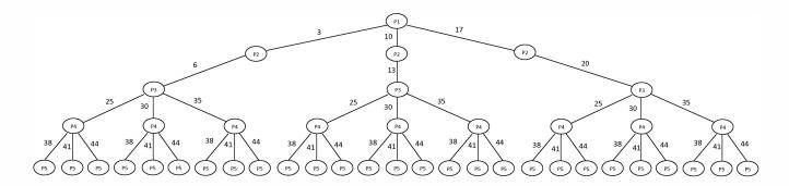
Fig. 1: An example path tree traversed by the recursive backtracking agorithm.
