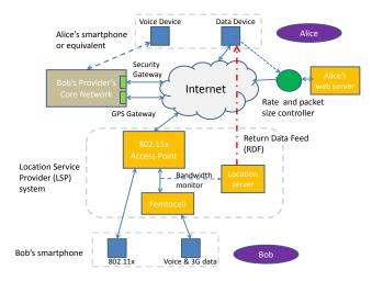
Fig. 1. Architecture of a single-carrier location authentication system.
